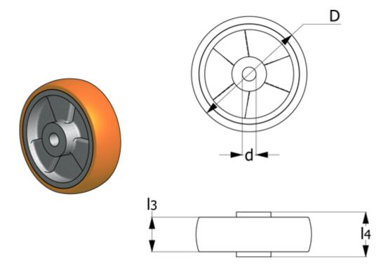
Code = 451516d = 20D = 150Dynamic load (N) = 6000I3 = 40I4 = 50Max static load (N) = 8500Rolling resistance (N) = 3300 Type = RE.F5-150-RSL Weight (g) = 910
